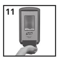
Place hand in middle of bar and push multiple times to prime refill. Product will dispense as bar is depressed.
