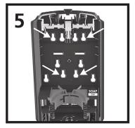
Using the dispenser as a template, pierce the tape on the back plate to mark and drill four holes using 1/4" drill bit. Use the supplied wall anchor and #10 x 1" screws to secure the dispenser in place, being careful not to over tighten. It is recommended to use 4 screws. If only two are possible, the top two holes should be used.
