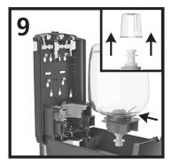
Remove refill cap and push the new refill into dispenser.
