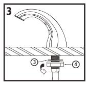
From underneath the counter, first feed the lock washer ③ and then the mounting nut ④ over the data cable ⑥ and onto the threaded stem of the dispenser-assembly ①. Be sure that the "teeth" on the washer will touch the bottom of the counter top and that the nut threads easily onto the stem. (If the nut is hard to turn by hand, it is upside down.) Hand-tighten the nut securely.
