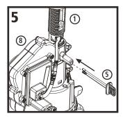
Secure the motor assembly/bottle support ® to the dispenser assembly ① stem by pushing the retaining dlp ③ into place through the vertical slots, until it goes all the way through the motor assembly.
