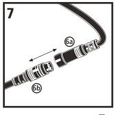
Connect the two halves of the data cable (6a) and (6b) by lining up the white stripes on each half and pushing the cable connectors together until the stripes touch.
