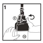
Grasp the empty refill bottle (1) with one hand and use the other hand to push the green release latch on the motor assembly/bottle support (2) to the right (counterclockwise as seen from above).
