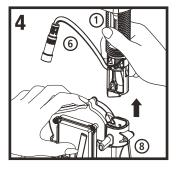
Align the indent inside the top of the motor assembly/bottle support (a) with the indent on the stem of the dispenser assembly (b) and firmly push the motor assembly/bottle support up, onto the stem.
