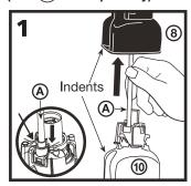
Snap in dispenser straw (A) (see inset). Feed the dispenser straw (A) on the refill bottle (10) up through the motor assembly/bottle support (8) and dispenser assembly (1), aligning the two indents in the bottle and the support. Slide the bottle upward until it snaps into place.
