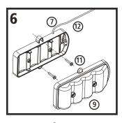
If using a battery box (a) remove the cover by loosening the two captive screws. Position the box on a convenient (vertical or horizontal) surface under the counter top that will allow access for battery changing. Attach the box to the surface using the two screws (1) and anchors (if attaching to a plaster or masonry surface). Use the wall clip (not included) to secure the power cable (1) to a wall or other under-counter surface if desired.
