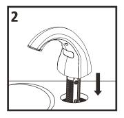
Feed the data cable (a) and the stem of the dispenser assembly (1) through the hole in the countertop. Point the spout of the dispenser into the sink bowl and press down firmly on the dispenser to securely attach it to the counter top.
