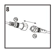
Connect the Power Connector to battery box or AC adaptor.
