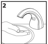
Test the system by passing your hand under the spout of the dispenser assembly ① (in front of the sensor window) three
