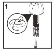
Remove the paper liner from the bottom of the adhesive gasket ② to expose the adhesive.
